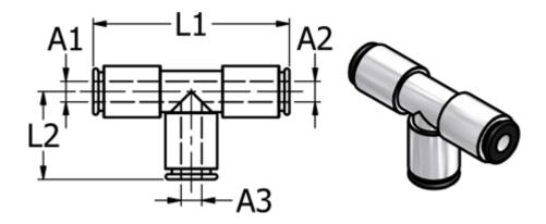
Ext. hose diameter A1 = 6Ext. hose diameter A2 = 6Ext. hose diameter A3 = 6L1 = 28 L2 = 19
